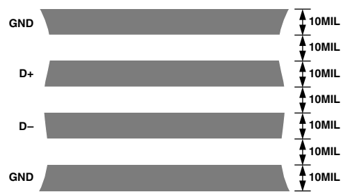
Figure 6. Arrangement of Signal Tracks
